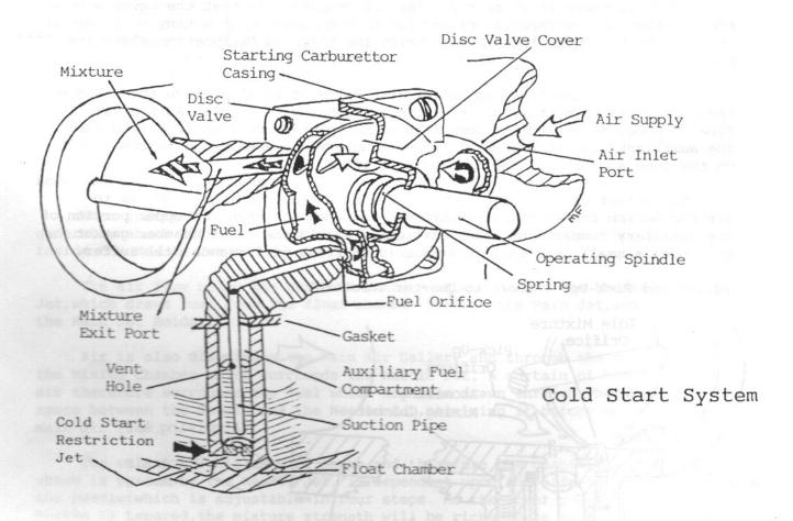
Rotation of the engine draws air into the Starting Carburettor, and through the exit port of the hollow disc valve. As it passes through, a vacuum is produced within the disc, which draws petrol from the float chamber via the orifices in the inner section of the disc. The atomised fuel therefore mixes with the air, and is drawn into the cylinder.
