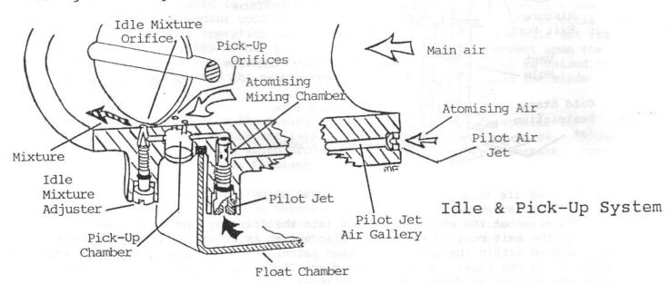
As the engine rotates, a vacuum is formed behind the closed throttle; this draws fuel from the float chamber and through the Pilot Jet, and into the atomisation chamber formed in the upper portion of the jet body, where it is
