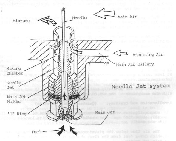
Should the Needle position produce too rich a mixture, the effect will be noted over a wide range of engine speed and load conditions as a general roughness, while a weak mixture will be obvious in terms of hesitation and misfiring on load.
